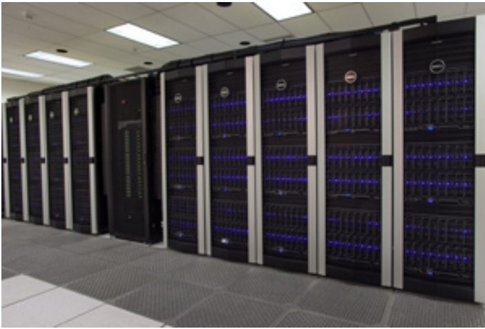
Deployed in February 2011, Lonestar 4 is TACC's newest supercomputer and the third largest system on the NSF TeraGrid. It ranks among the most powerful academic supercomputers in the world with 302 teraflops peak performance, 44.3 terabytes total memory, and 1.2 petabytes raw disk.
